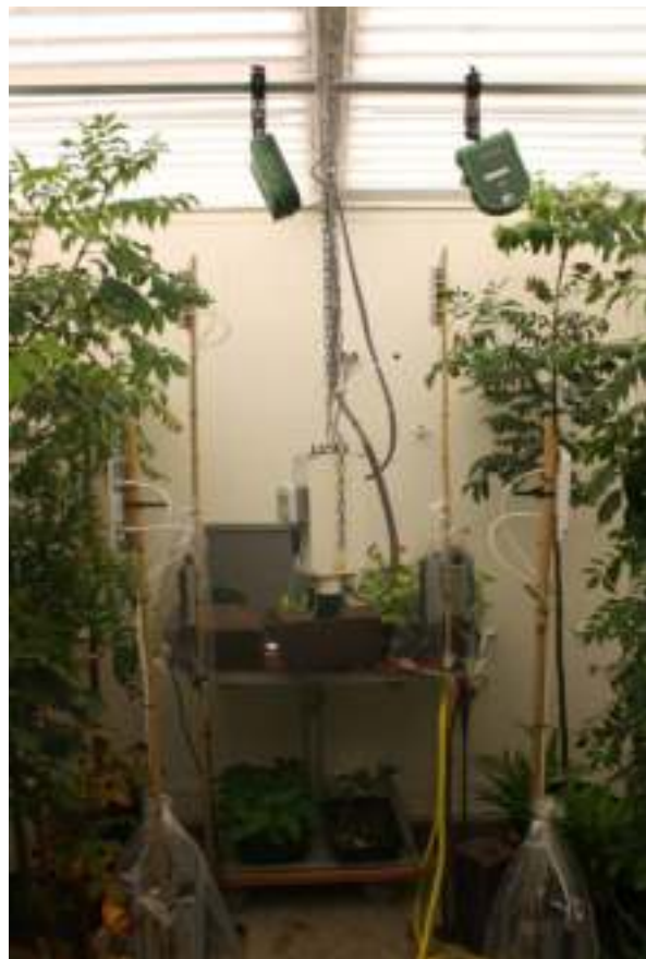
Photo 4: Overall set-up in the climate chamber including the Wifi routers and the antenna's
